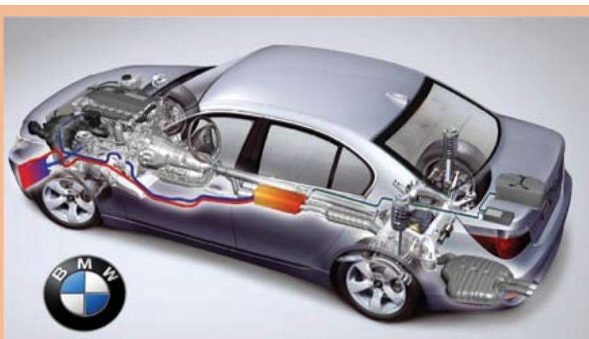
FIG. 2. Conceptual design of thermoelectric generator producing electricity from waste heat in the engine exhaust. Copyright BMW, reprinted by permission.
